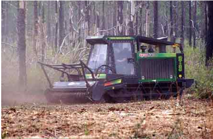
Figure 14. Using gyrotrac to clear heavy brush on Unit #4.
